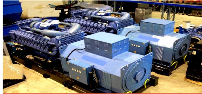
Generators Coupled to MTU Engines
