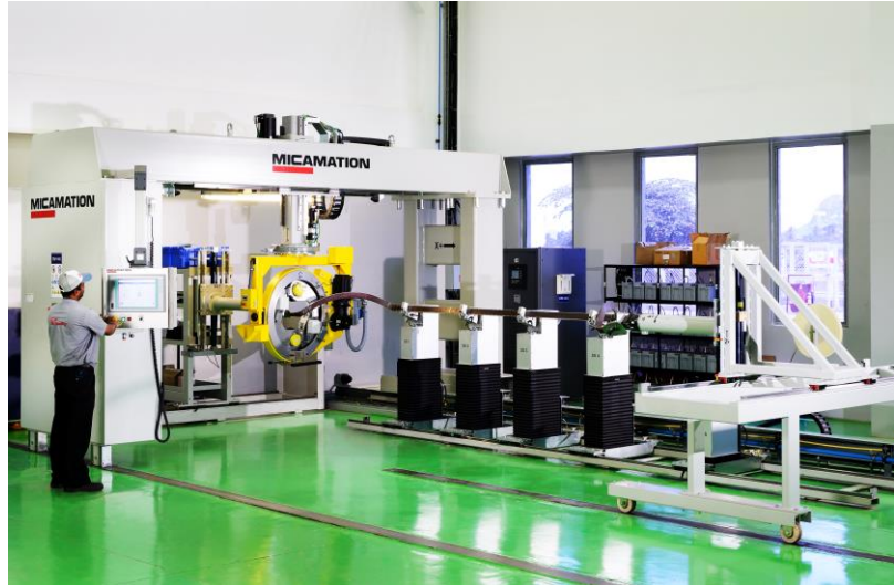
Automatic Taping Machine, Micamation Switzerland Maximum Bar Length With Overhang – 6000mm
