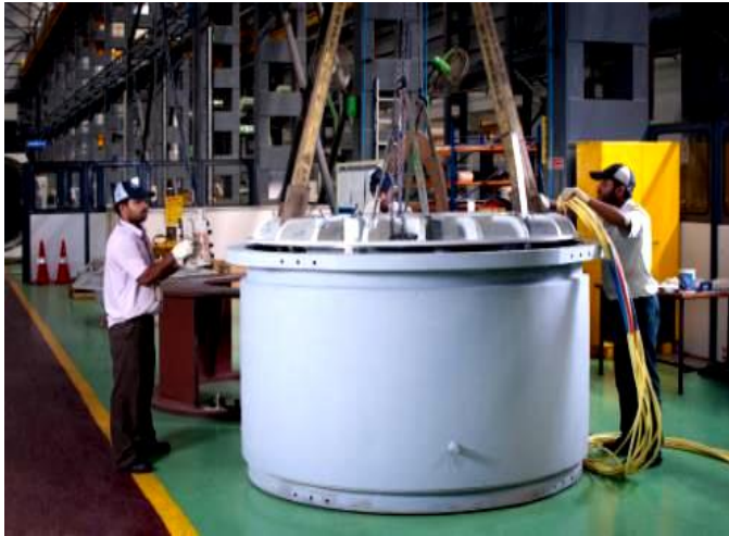
1MW, 144rpm / 138rpm Permanent Magnet Generator
